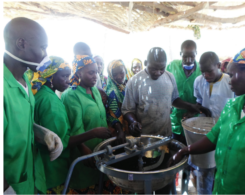
Photo 3a: Mixing components with the binder to produce biofuel pellets Photo credit: Fadimatou Hassimi (Association Horizon Info)
