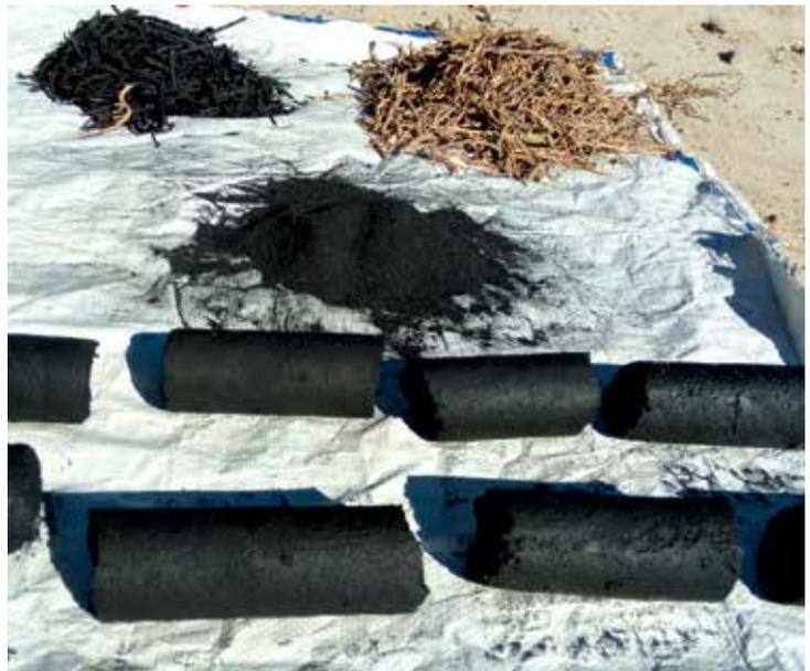
Raw materials (stems and rosemary leaves), carbonization product (dust), powder obtained after grinding and compressed and dried briquettes. Morocco.
