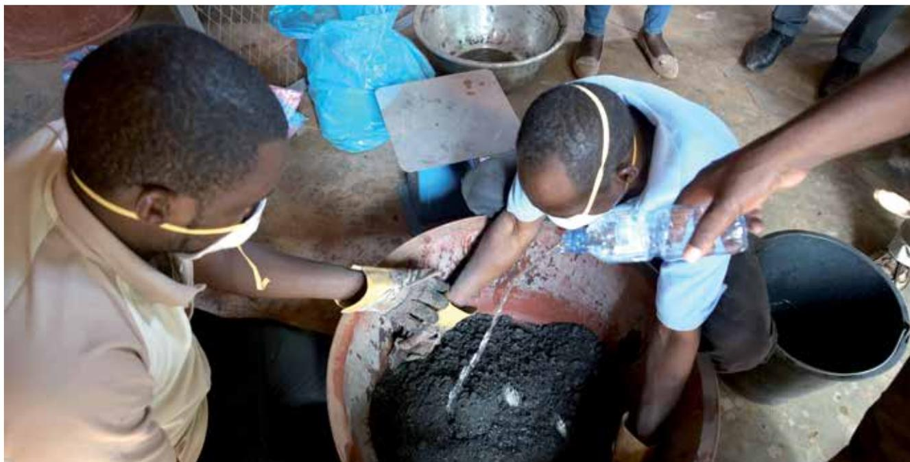
Added binder to powder after carbonization and grinding. Burkina Faso.
