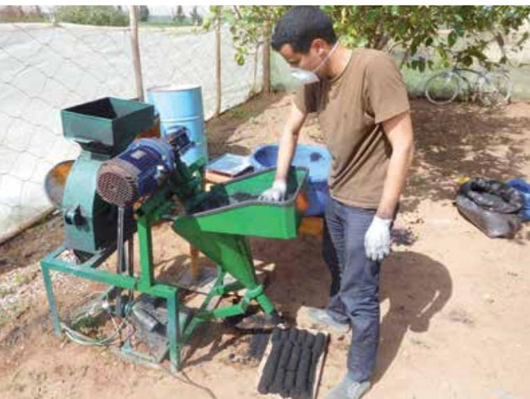
Material that performs two operations: grinding and compacting. Morocco.
