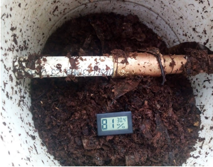
Figure A3: Photo showing inside of a UCU in use, with humidity and temperature recorder
