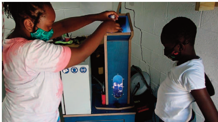
Loading machine to make upcycled plastic products (Photo courtesy WISH Foundation)
