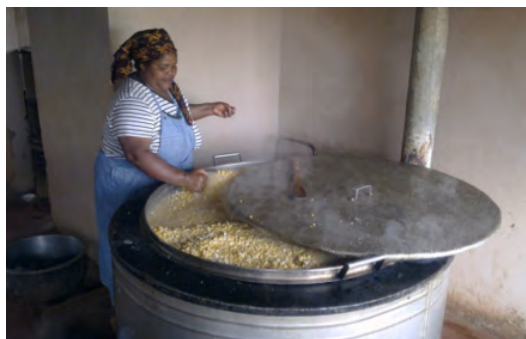
Picture 1. Efficient stove for institutional use, Kenya
