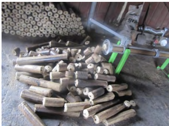
Picture 4. Biomass briquettes production, Romania
