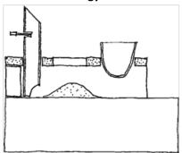
The CETA modified eco-stove features two burners and a chimney and is effective for pots of up to 12 litres capacity. It works especially well for foods that require direct heat such as rice. This stove model, which costs about \$44, is widely used in rural Nicaragua, Guatemala and El Salvador. It is mainly built from simple materials such as clay, bricks, cast iron, cement, metal, and mud. Achieving high fuel economy and reductions in
