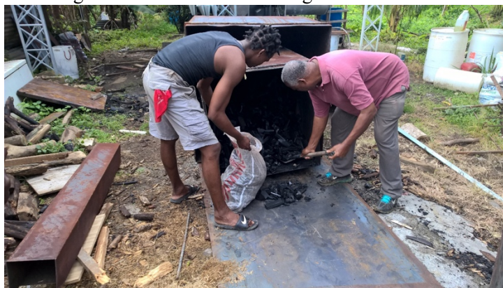
Photo 2: Removing biochar from the unit @ GOAM
