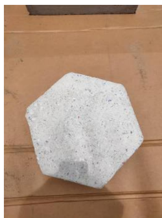
Picture 10: Ground dirty, waste plastic found on beach Picture 11: Participants shovelling the concrete and plastic mix from the ransom into the paver mould. Picture 12: An example of the completed product. Picture 13: Bench and pot donated by FTEM and now on Moruga Beach.
